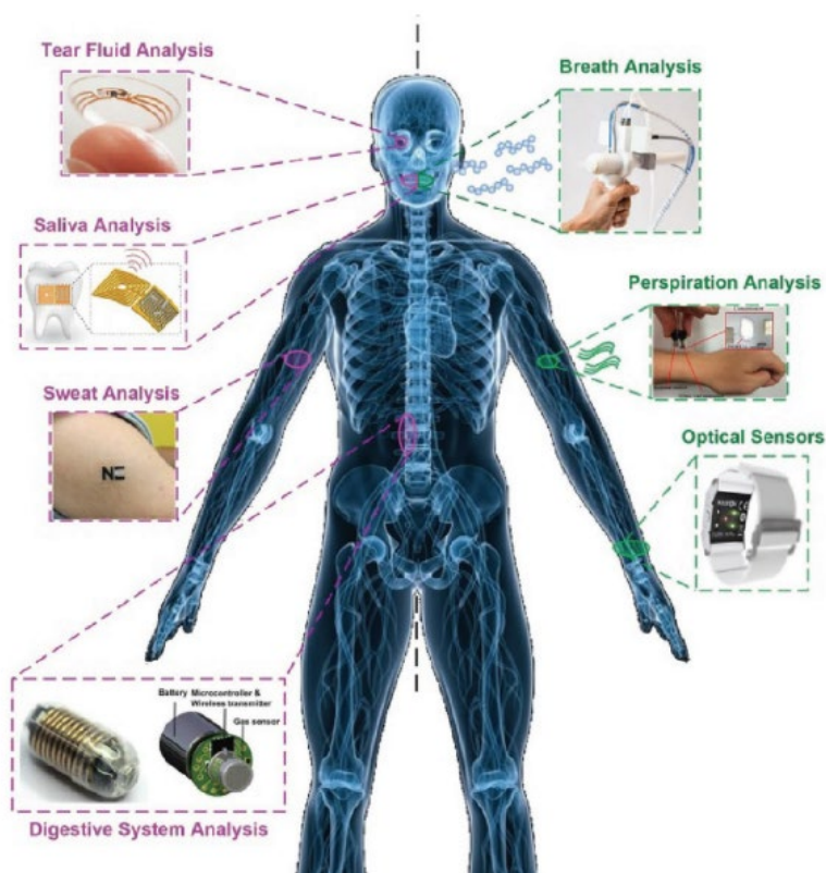
Figure 1: Schematic summary of some emerging sensing technologies for personalized and preventive medicine. A major distinction can be made between contact and contactless technologies, such as tear, saliva analysis, sweat, digestive system and optical, breath and perspiration analysis [1].
