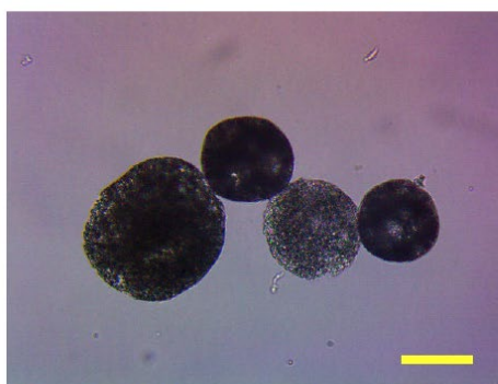
Figure 1: Optical microscope image of gigaporous microparticles, scale bar is 70 μm.
